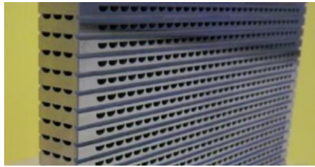
Figure 2 Semi-circular cross-section shape PCHE
