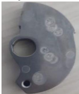
Figure 11 - Image of the part after metallographic testing done on the spectrophotometer machine.
