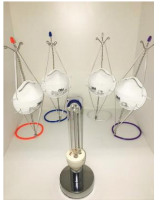
Figure 2 - Image of the interior of the cab with lamp and N95 masks positioned
