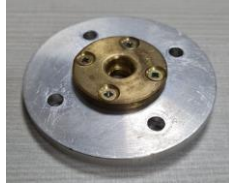
Figure 16. High base parts and puncture guide joined by screws
