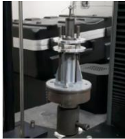
Figure 19. Device being used in spring testing.
