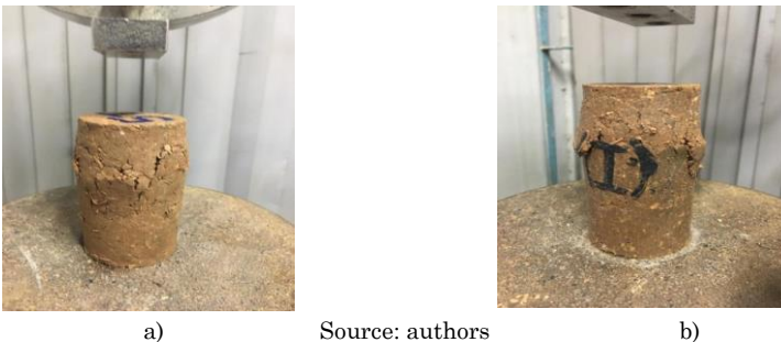
Figure 05: a) Breakage of the test specimens of composites S70R27M3 and b) S50R47M3
