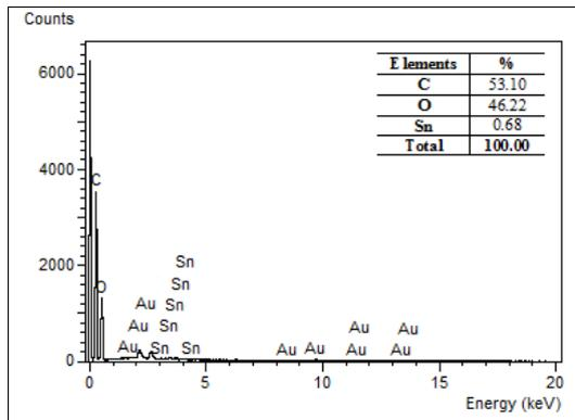
**Figure 3 – Spectrum by EDS analysis [2].**
