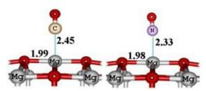
**Scheme 1**. Presentation of CO and NO adsorptions on the surface of the MgO nanotubes [2].
