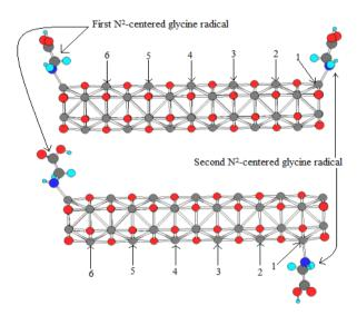
**Figure 9**. The interaction of the two radicals of glycine with the MgONTs, so that the two radicals are in same side (above) or in opposite side (below). The numbers show positions of the second radical of glycine, which must in each step toward the first radical, so that the first radical of glycine remain in the same position.
