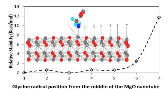
**Figure 7.** The relative stability of the  $N^2$ -centered glycine radicals with MgONT as a function of the position of the single covalent  $N_{Glycine}$ -MgMgONT bond that formed, from the middle of the MgONT toward their two ends.
