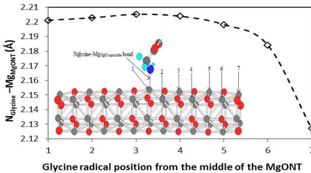
**Figure 8.** The  $N_{\text{Glycine}}-\text{Mg}_{\text{MgONT}}$  bond length as a function of the position of the single covalent  $N_{\text{Glycine}}-\text{Mg}_{\text{MgONT}}$  bond that formed, from the middle of the MgONT towards one of their two ends.
