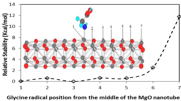
**Figure 7.** The relative stability of the  $N^2$ -centered glycine radicals with MgONT as a function of the position of the single covalent  $N_{\text{Glycine}}-\text{Mg}_{\text{MgONT}}$  bond that formed, from the middle of the MgONT toward their two ends.
