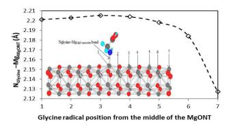
**Figure 8.** The  $N_{Glycine}$ – $Mg_{MgONT}$  bond length as a function of the position of the single covalent  $N_{Glycine}$ – $Mg_{MgONT}$  bond that formed, from the middle of the MgONT towards one of their two ends.
