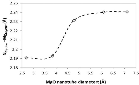
**Figure 4.** The N<sub>Glycine</sub>-Mg<sub>MgO</sub> bond as a function of MgO<sub>NT</sub> diameter.
