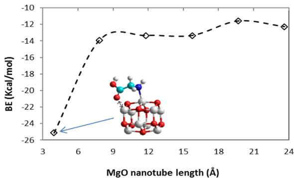
**Figure 5.** The binding energy of the N<sup>2</sup>-centered glycine radicals with the Mg<sub>MgO</sub>NT as a function of MgO<sub>NT</sub> length.
