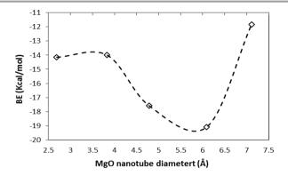
**Figure 3.** The binding energy between the  $N^2$ -centered glycine radical and the MgMgONT as a function of the MgONT diameter.
