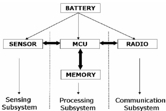
Figure 1: An overview of wireless sensor networks
